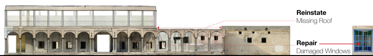
Block A & B Existing Elevation
